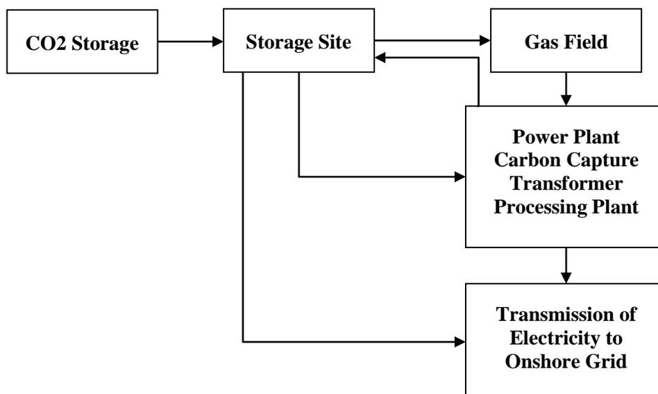
Figure 2-5: Design selection flowchart for CO<sub>2</sub> storage option
