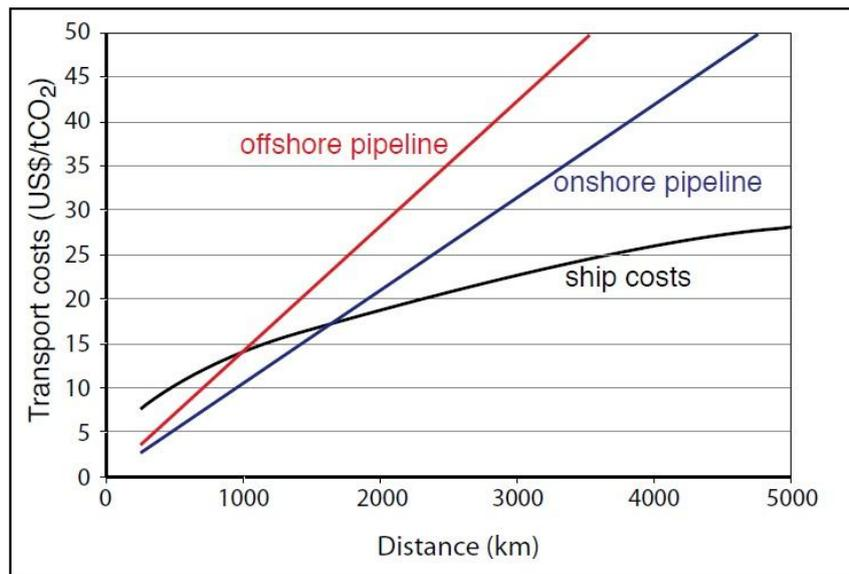
Figure 1-5: Cost estimate for CO<sub>2</sub> transport options (IPCC 2005: IPCC Special Report on Carbon Dioxide Capture and Storage. Prepared by Working Group III of the Intergovernmental Panel on Climate Change, Figure TS.6 Cambridge University Press)
