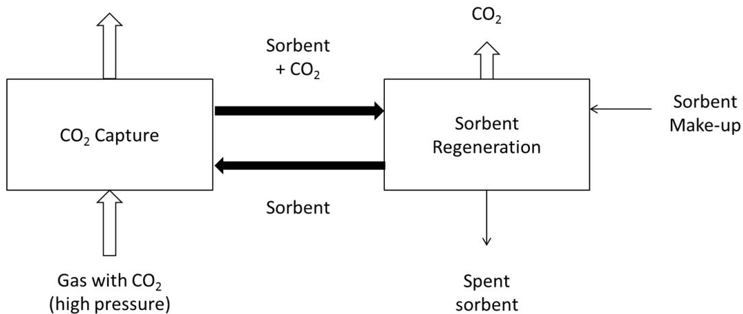
Figure 2-29: Physical absorption system
