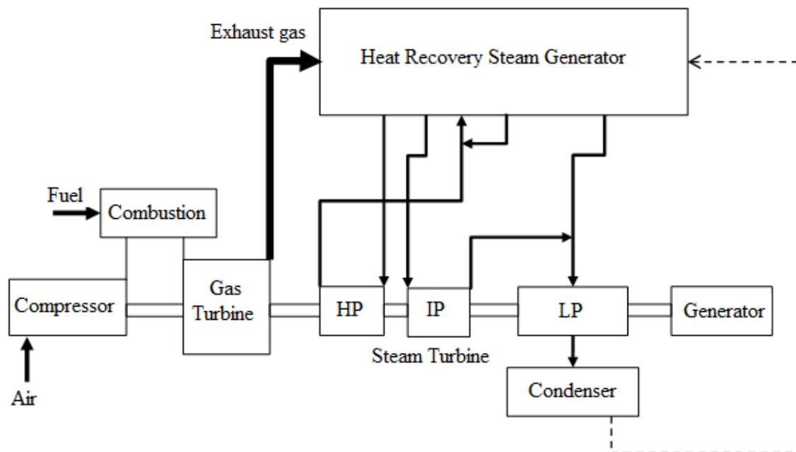
Figure 2-25: Combined cycle gas turbine
