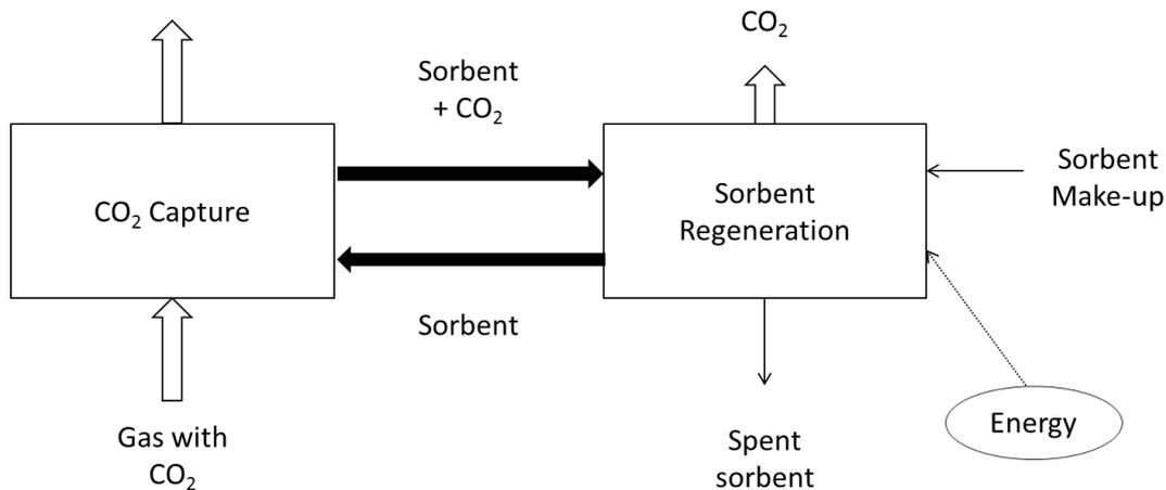
Figure 2-28: Chemical absorption system
