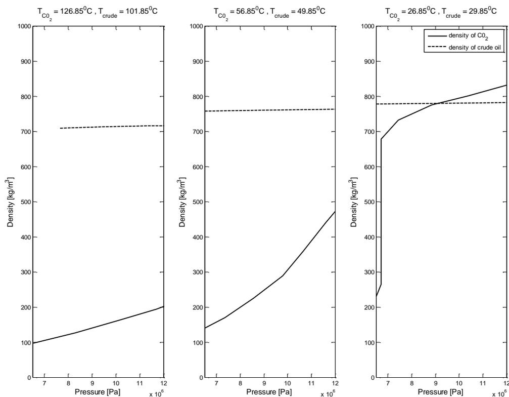
Figure 1-21: Comparison of CO<sub>2</sub> and North Sea crude oil densities at different temperatures and within the working pressure range of most pipelines
