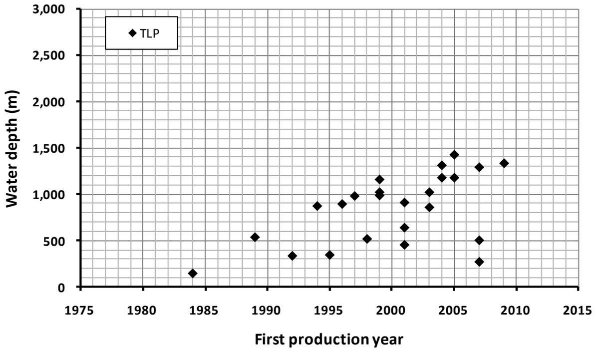
Figure 2-19: Relationship between first production year and water depth for TLPs
