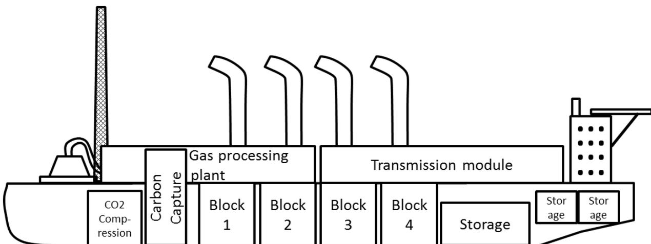
Figure 3-8: Layout of Offshore Thermal Power Plant (OTPP)
