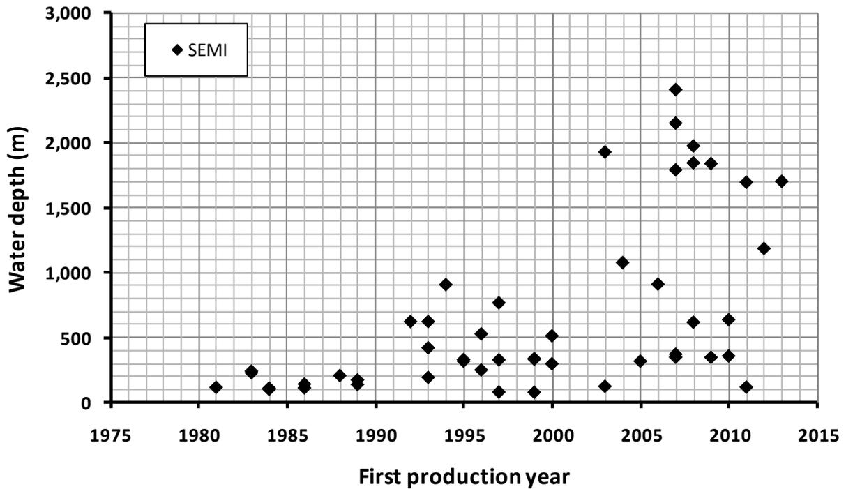
Figure 2-21: Relationship between first production year and water depth for semi-submersibles
