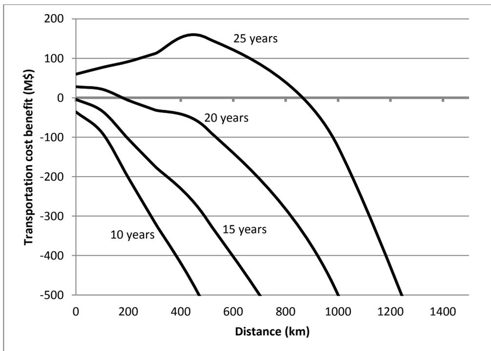
Figure 3-15: Cost reduction of GTW compared to conventional transportation at high estimation of cable cost
