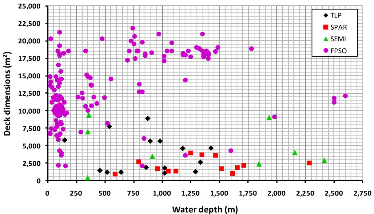
Figure 2-23: Relationship between deck area and water depth for different types of offshore structure
