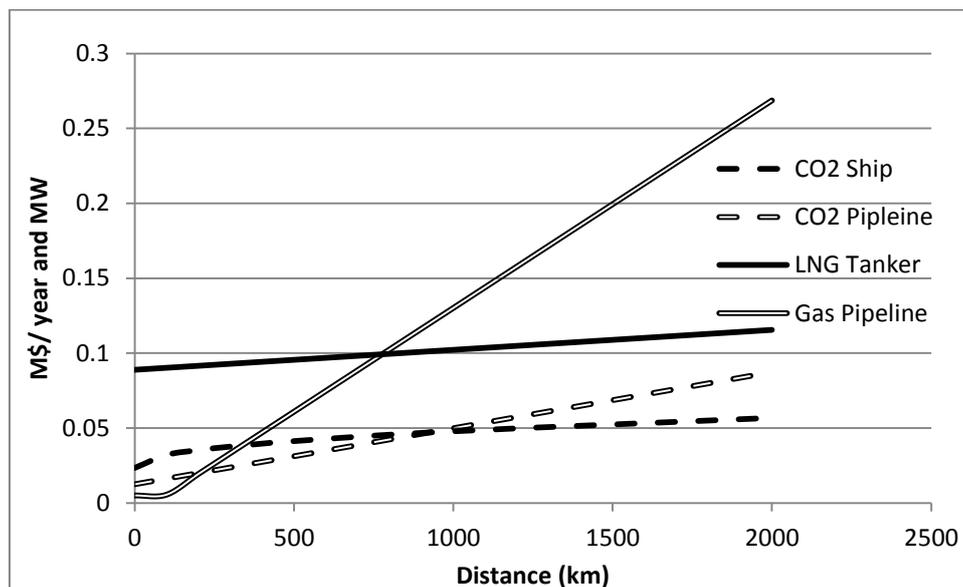
Figure 3-9: Estimate of transportation costs per year and MW for an onshore power plant
