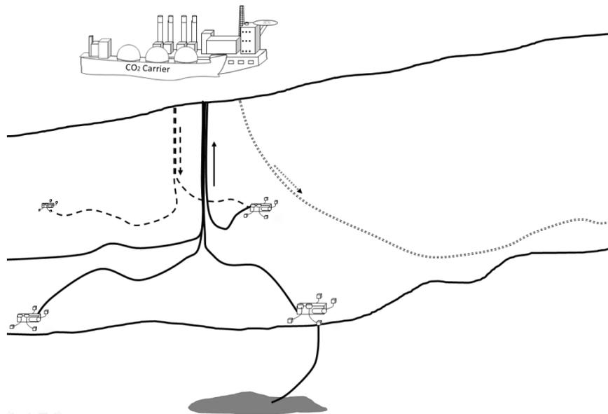
Figure 5-1: Schematic of CO<sub>2</sub> carrier utilising the injection capabilities of an offshore power plant
