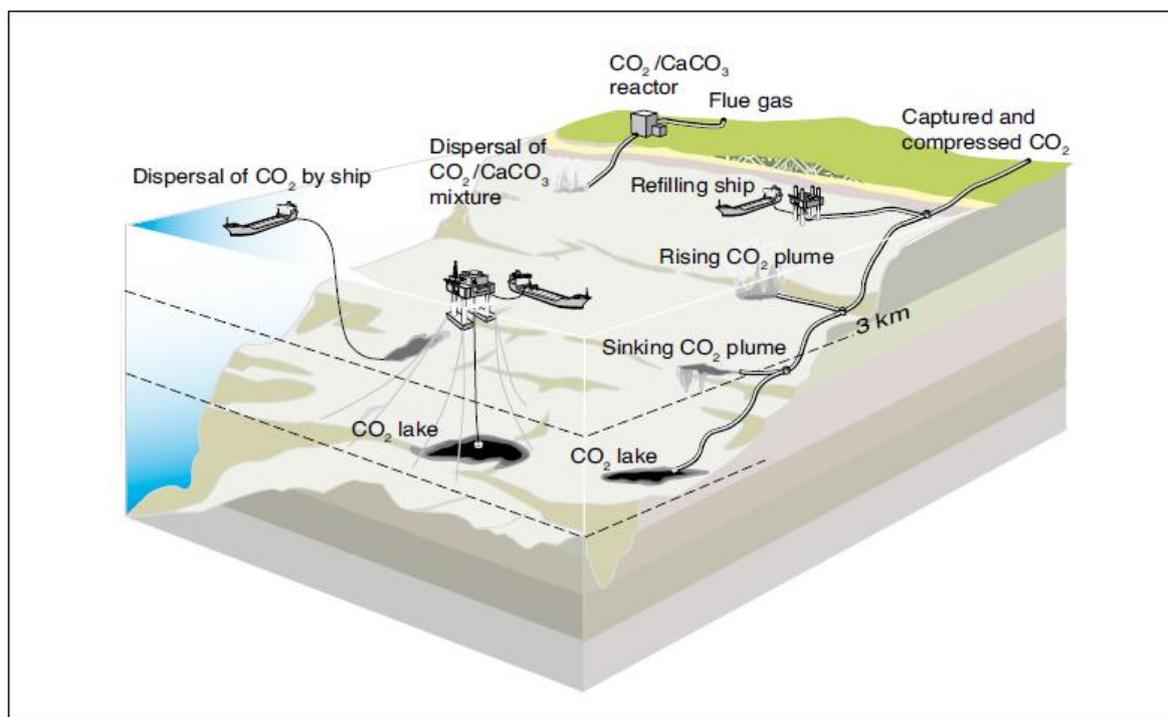
Figure 1-9: Methods of ocean storage (IPCC 2005: IPCC Special Report on Carbon Dioxide Capture and Storage. Prepared by Working Group III of the Intergovernmental Panel on Climate Change, Figure TS.9 Cambridge University Press)
