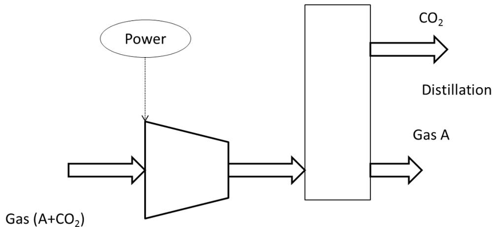
Figure 2-32: Cryogenic system
