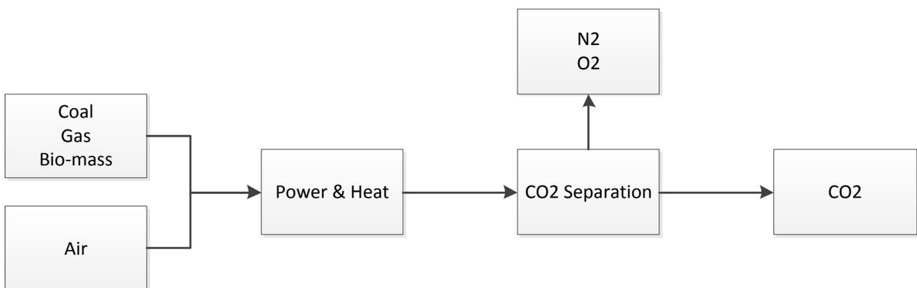
Figure 1-3: Post-combustion process flowchart
