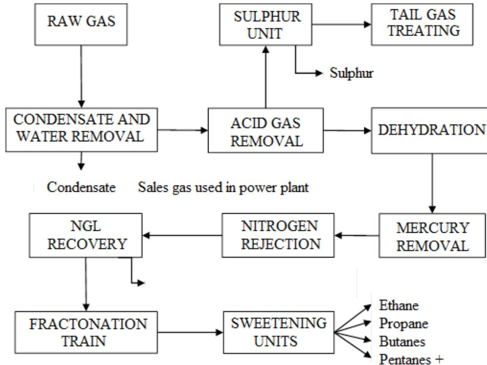
Figure 2-26: Typical Natural Gas processing flow diagram
