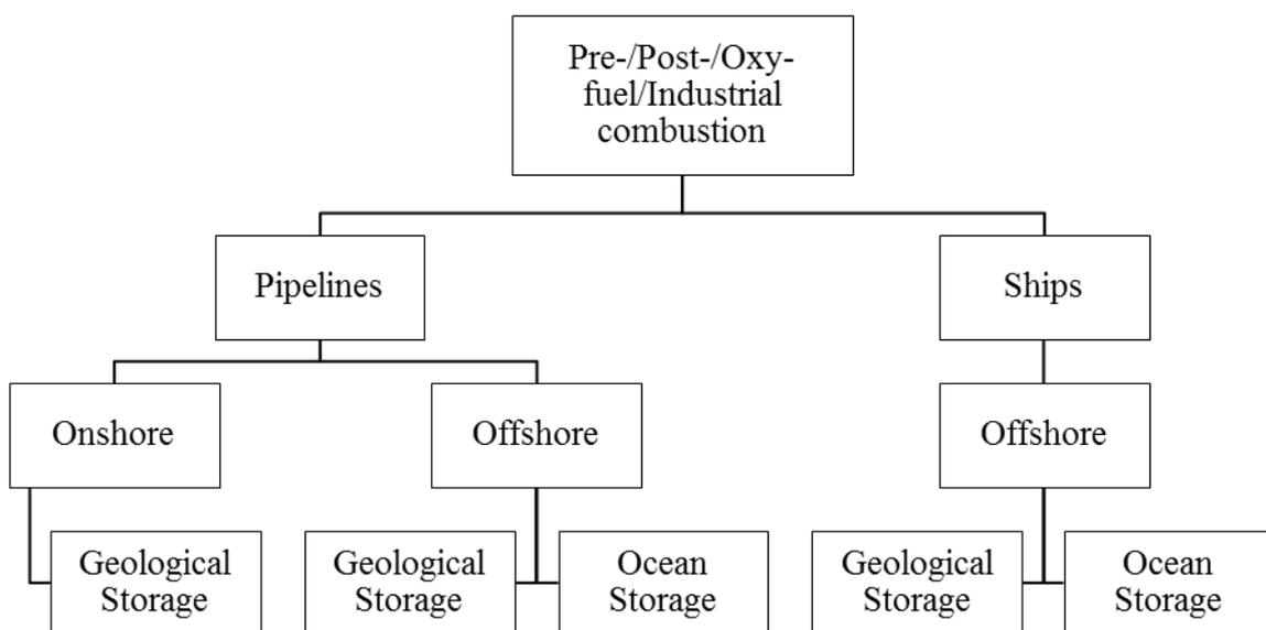
Figure 1-1: Carbon Capture & Storage flowchart
