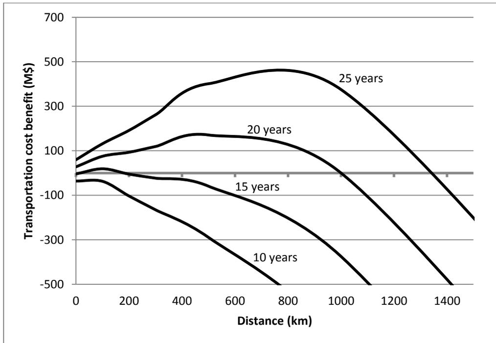
Figure 3-14: Cost reduction of GTW compared to conventional transportation
