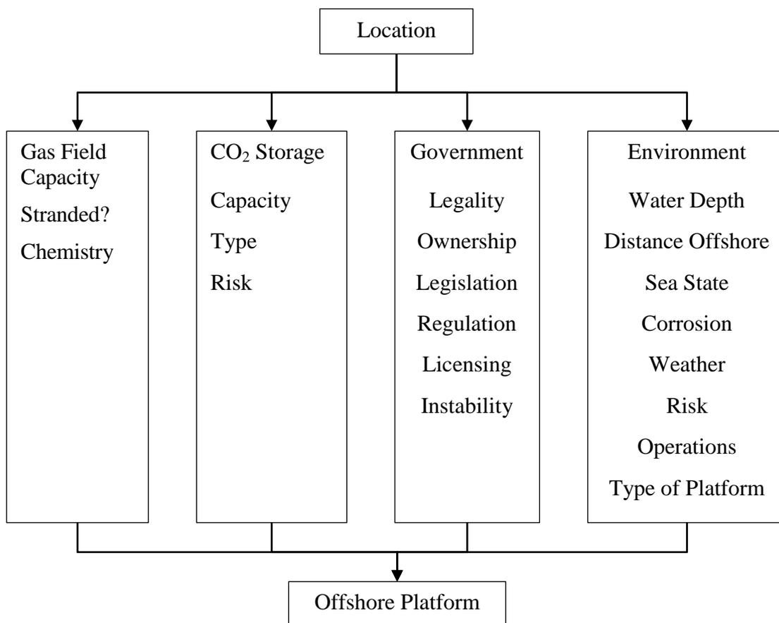
Figure 2-6: Factors affecting design of offshore power plants
