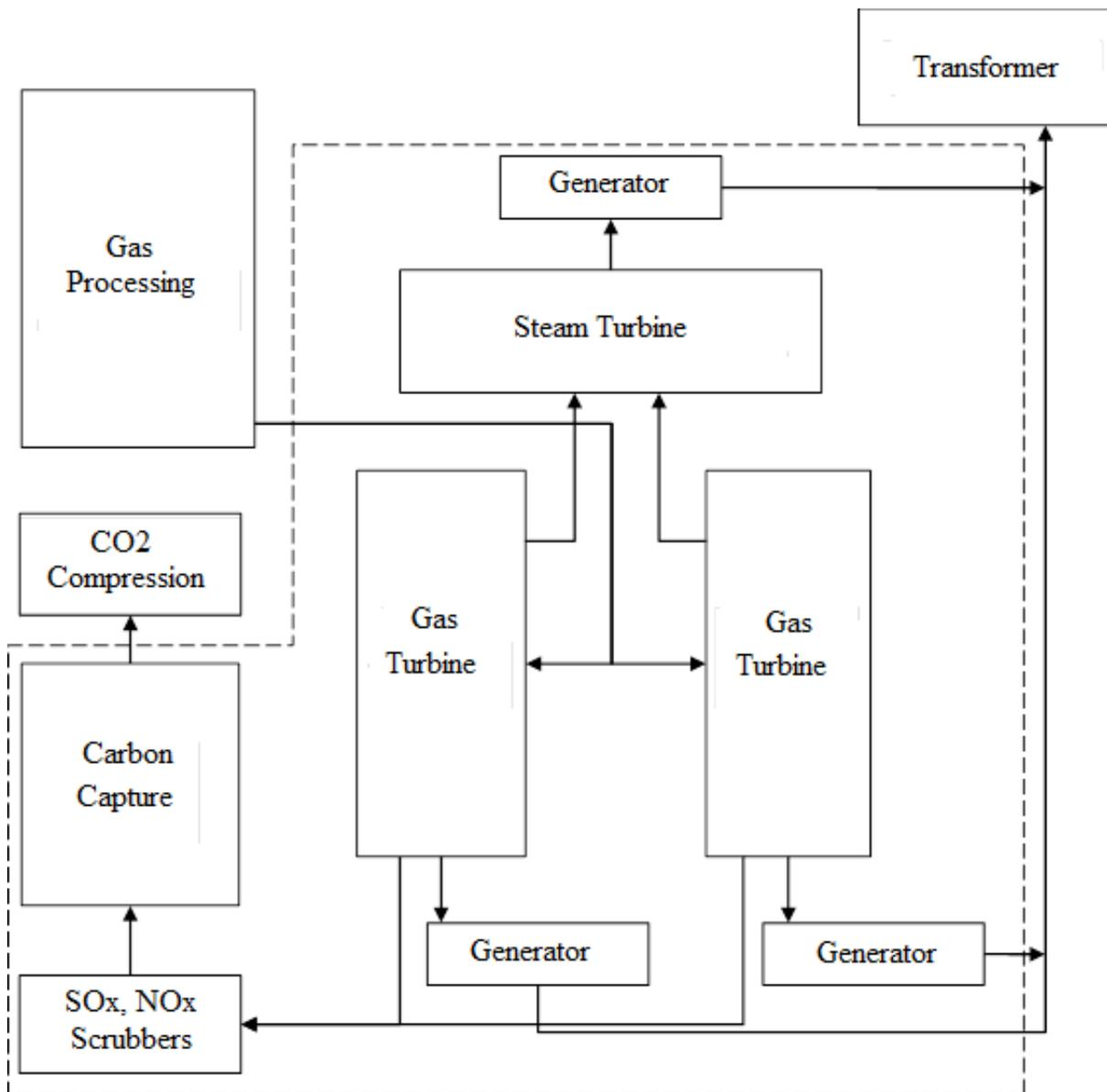
Figure 3-6: Arrangement of one Power Generation Block
