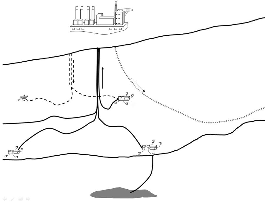
Figure 2-24: An Offshore Power Plant served by local subsea installations and a more distant source
