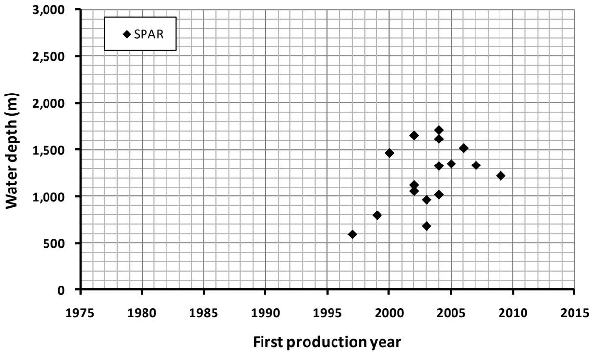
Figure 2-20: Relationship between first production year and water depth for spars
