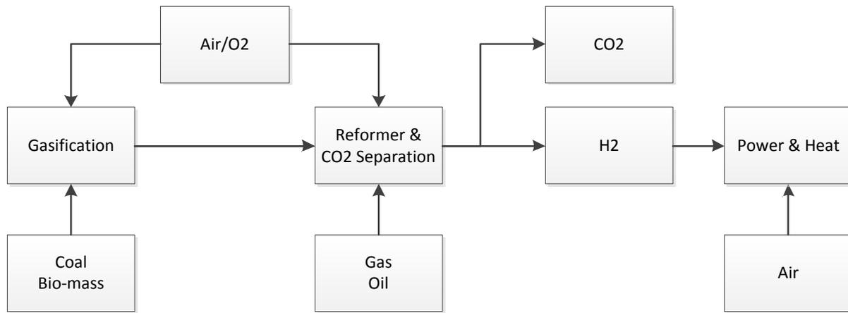
Figure 1-2: Pre-combustion process flowchart
