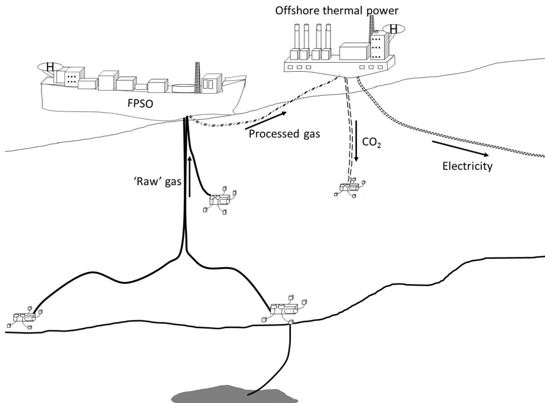
Figure 2-2: Schematic of offshore thermal power with FPSO
