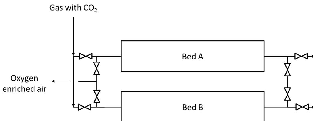
Figure 2-30: Adsorption system (PSA)
