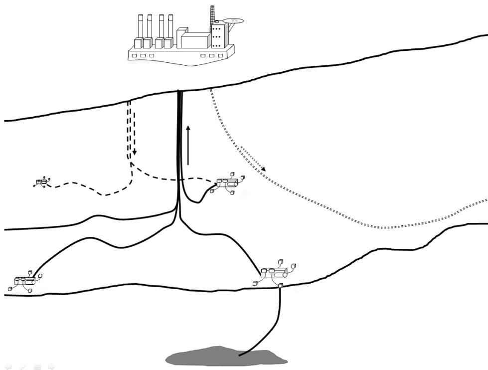
Figure 2-1: Schematic of offshore thermal power with CCS
