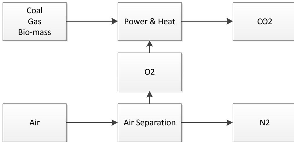
Figure 1-4: Oxy-fuel process flowchart
