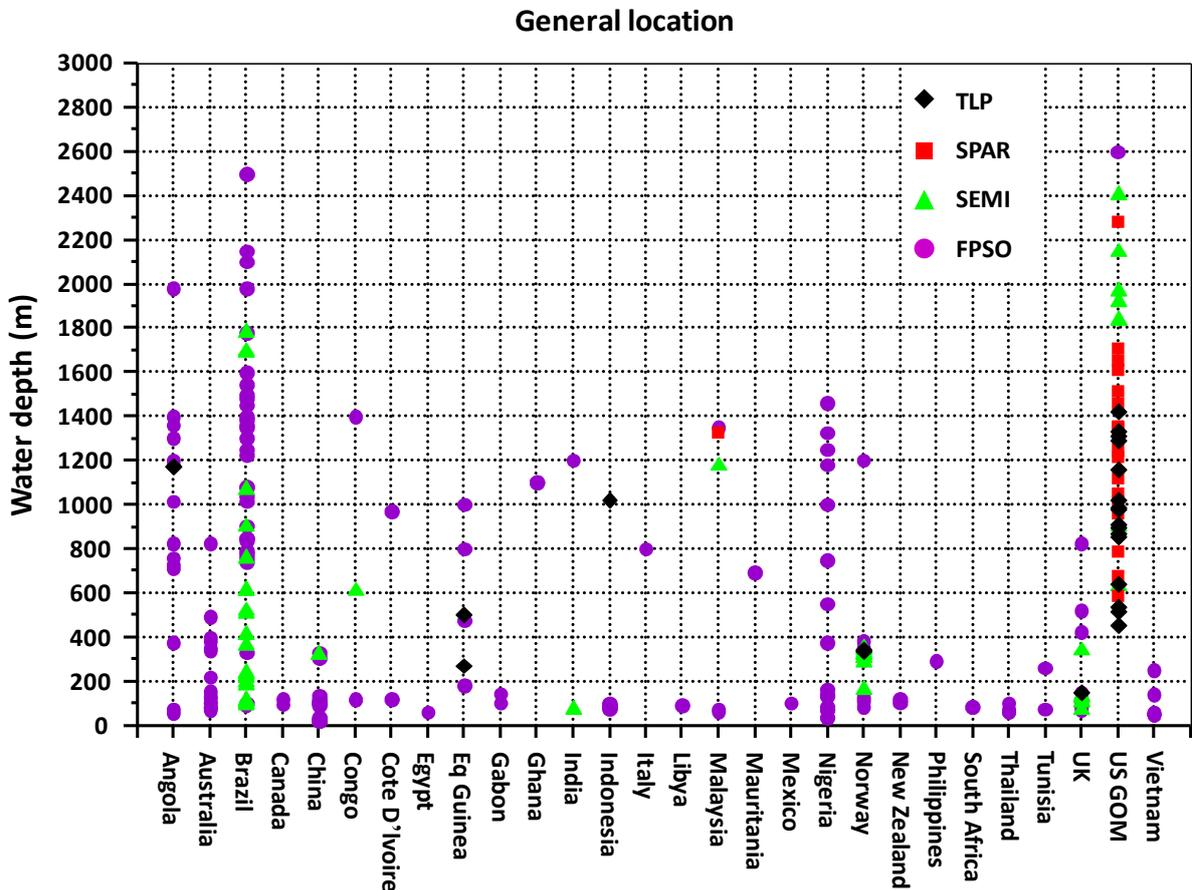
Figure 2-14: Relationship between general location of oilfield and water depth
