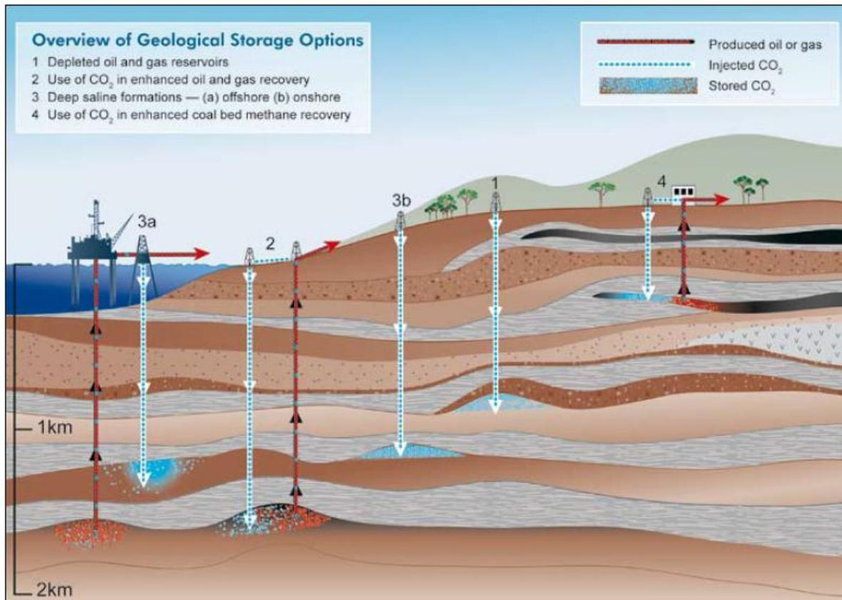
Figure 1-8: Methods for storing CO<sub>2</sub> in geological formations (IPCC 2005: IPCC Special Report on Carbon Dioxide Capture and Storage. Prepared by Working Group III of the Intergovernmental Panel on Climate Change, Figure TS.7 Cambridge University Press)
