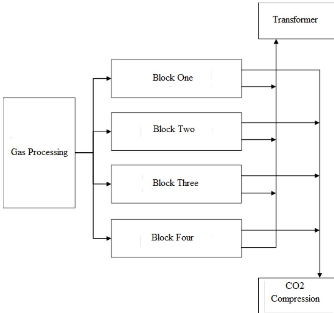
Figure 3-7: Arrangement of the four Power Generation Blocks
