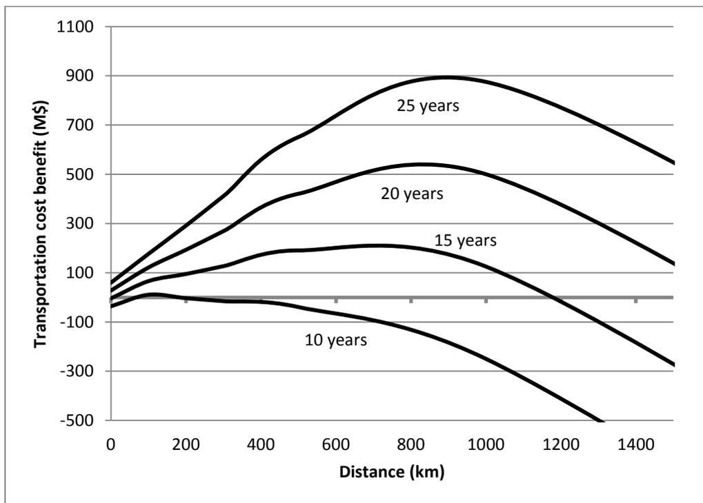
Figure 3-16: Cost reduction of GTW compared to conventional transportation at low estimation of cable cost
